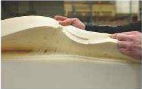
Foam Assembly with HMPSA
