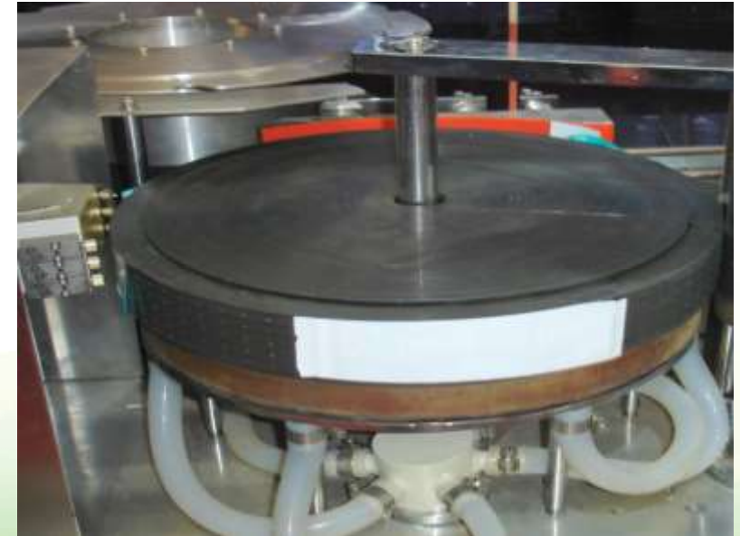
Labelling Process – Nozzle Based
