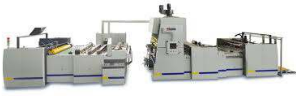
Typical Dry Lamination m/c using Water based Adhesives
